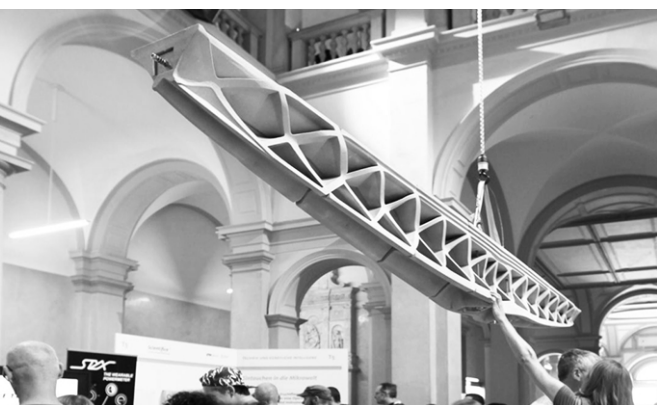
FIGURE 9 3D Printed Reinforced Beam from ETH Zürich, https://dbt.arch.ethz.ch/project/3d-printed-reinforced-beam/ , accessed on 27.07.2022
